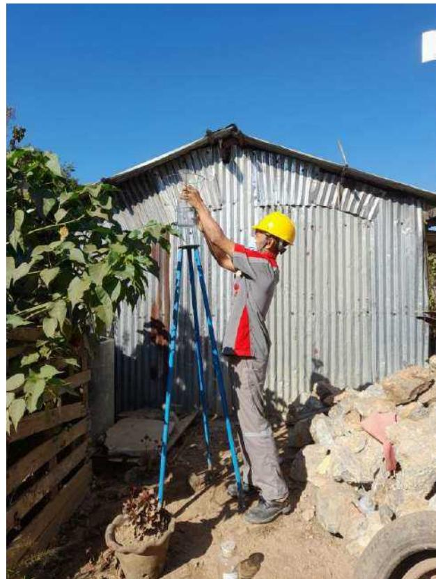
Figure8 – Dust Deposition Monitoring
